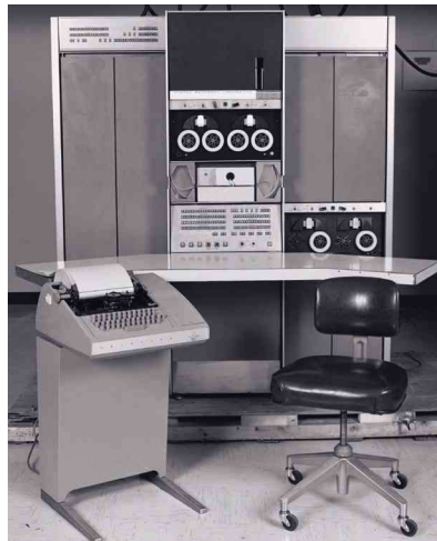
Figure 2.1 A minicomputer similar to Thompson's PDP-7. 52
